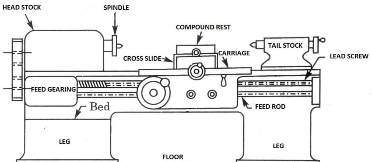
Lathe machine tool
